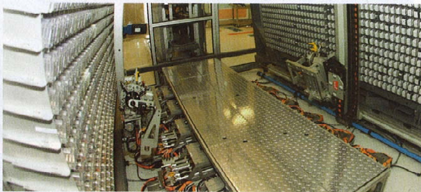
A 50-foot-long, 20-foot-wide conveyor-style robot plucks the blisters, each with its own bar code, from the tubes and puts them in sealed pouches. It can fill 465 patients’ daily regimens—including four dispensing rounds of up to 12 different medications—every hour.
